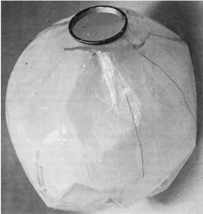
Fig. 1. Liquid-propellant expulsion bladder which has failed from tears and cracks near the aluminum seal ring.
